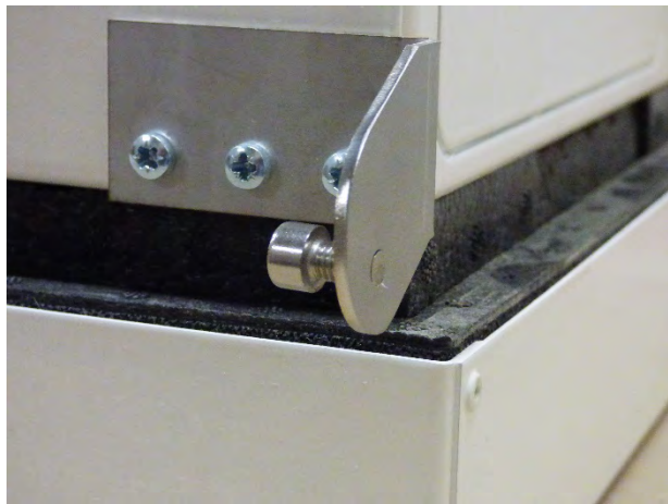
Figure 18 Bottom hinge bracket with screw not protruding
