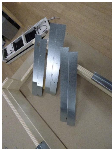
Figure 9 Break U shape into 3 pieces
