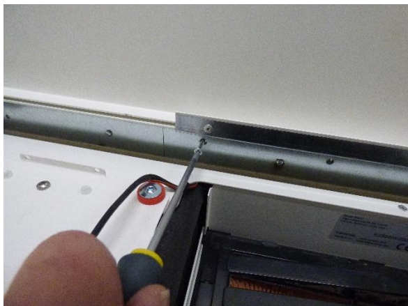
Figure 44 Secure door frame at each side with screws provided
