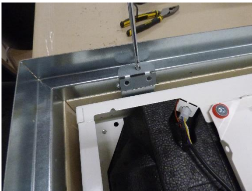
Figure 27 Mounting bracket formed and fixed with screw in dedicated hole
