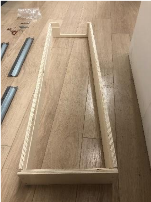
Figure 4 Timber frame screwed together
