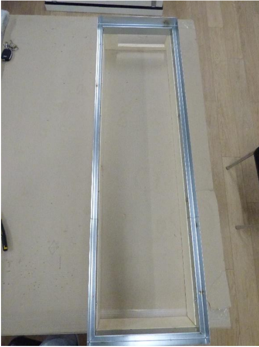
Figure 8 Fit the two middle strips so that all edges do not overlap
